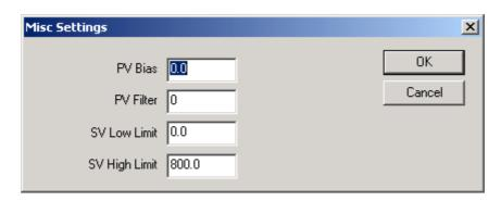
Enter the values for PV Bias and Filter and SV Limits, Click OK to write the data to the controller.
