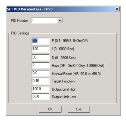
Select a PID Number, enter the PID parameters as required, Click OK to write the data to the controller.
