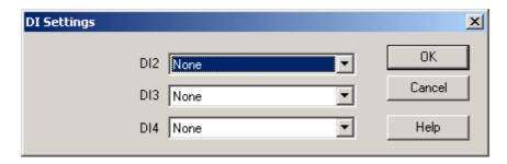
Select the mode for DI operation, Click OK to write the data to the controller. When a DI mode is set, that operation cannot be performed via the software. i.e if DI is set to Auto Tune, Auto Tune cannot be started via the software.
