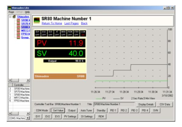
The controller is shown along with the graph showing recent values of PV and SV of the controller.
