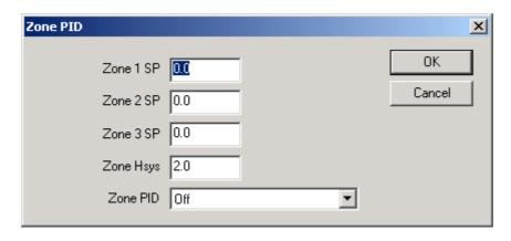
Enter the Zone PID parameters as required, Click OK to write the data to the controller.
