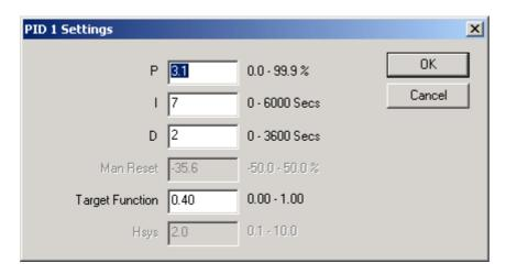
Enter the PID parameters as required, Click OK to write the data to the controller.
