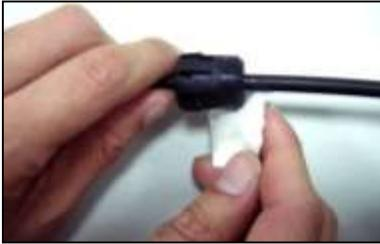
Clean fiber and the surface of fiber with alcohol.
