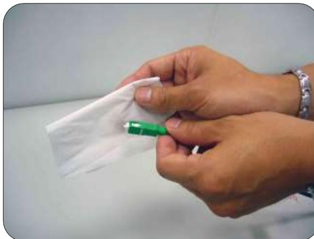
Apply the alcohol onto the Kimwipes and
