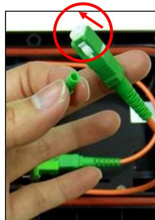
Remove the cap of the connector
