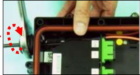
Tighten the cap in a clockwise way with spanner
