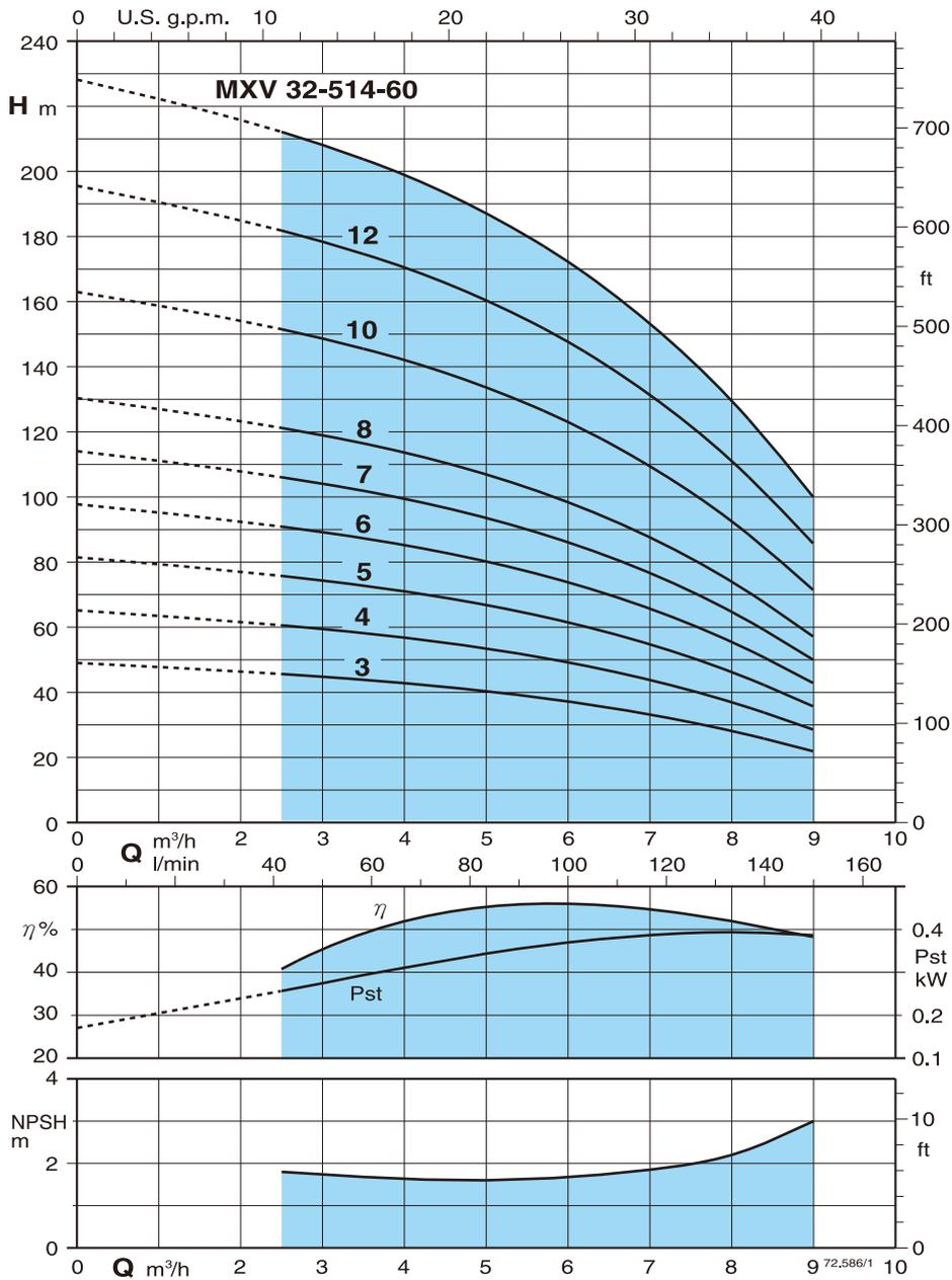
Test results with clean cold water, without gas content.
