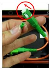
Remove the cap of the connector
