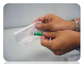
Apply the alcohol onto the Kimwipes and clean the SC/ APC connectors thoroughly. Take note as not to touch the wet part of the Kimwipes with your hand
