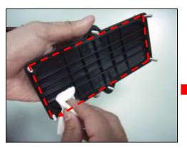
Clean the O-ring and the joint of the upper cover with alcohol.
