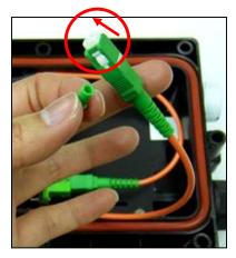
Remove the cap of the connector
