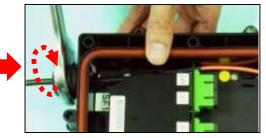
Tighten the cap in a clockwise way with spanner
