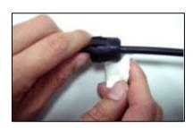
Clean fiber and the surface of rubber with alcohol Tighten the cap in a
