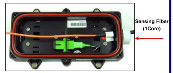
Step 2 Remove the cap of the adaptor.
