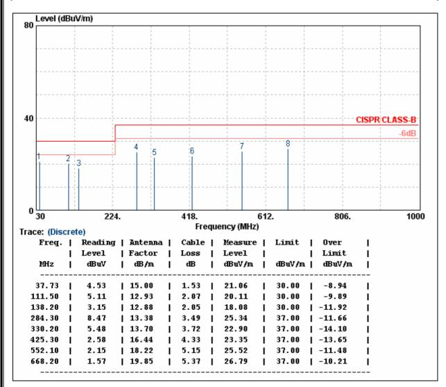
REMARKS: 1.Level (dBuV/m) = Read Level (dBuV) + Antenna Factor (dB/m) + Cable loss (dB) 2.Over Limit value (dB) = Level (dBuV/m)-Limit Line(dBuV/m)
