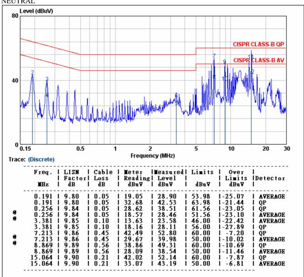
REMARKS: 1.Level (dBuV/m) = Read Level (dBuV) + Antenna Factor (dB/m) + Cable loss (dB)2. Over Limit value (dB) = Level (dBuV/m)-Limit Line(dBuV/m)
