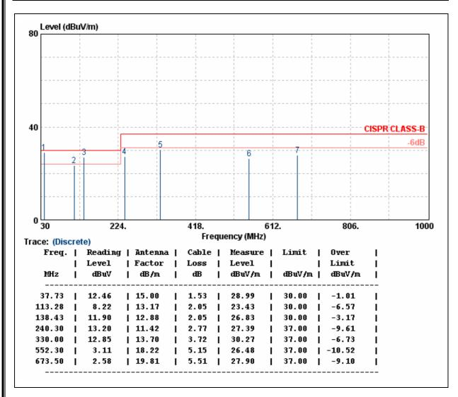
$REMARKS: \quad 1.Level \ (dBuV/m) = Read \ Level \ (dBuV) + Antenna \ Factor \ (dB/m) + Cable \ loss \ (dB)$
