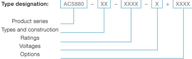
has a unique type designation, which identifies the drive by construction, power and voltage range. The options are added to the type designation with a "plus" code. Build up your own ordering code using the type designation key or contact your local ABB drives sales office and let them know your needs/ requirements.
