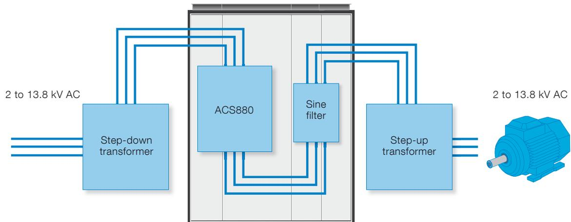
For step-up applications eg, where medium voltage motor needs to be driven
